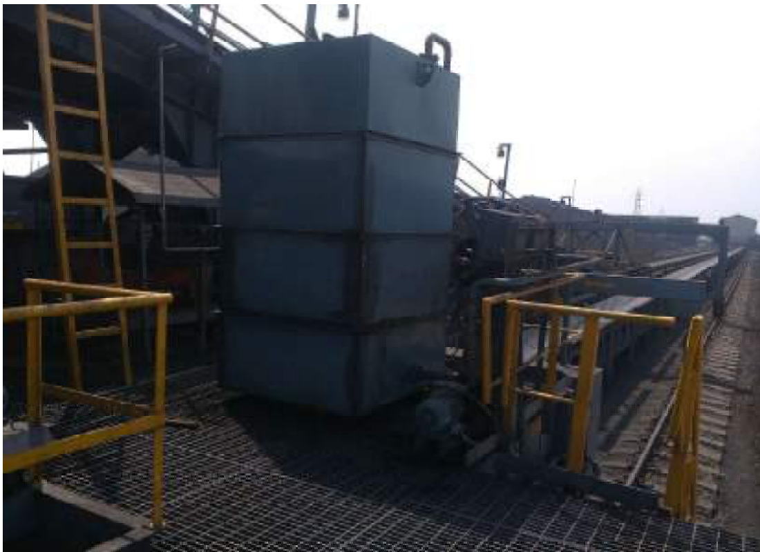
High efficient in build water sprinkler system provided in the staker/reclaimer
